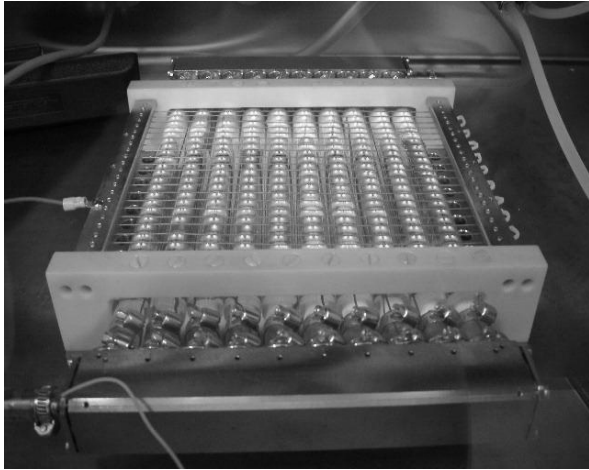
Fig. 7. Excilamp's photo in working mode
